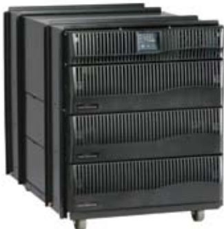
Powerware 9125 6000 VA with 2 EBMs
